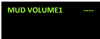
Figure 6. Readings in case of loss of communication with the U-150
