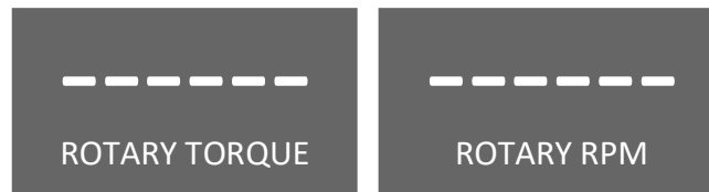
Figure 19. Readings on a screen of control module if there is a loss of connection with an indicator
