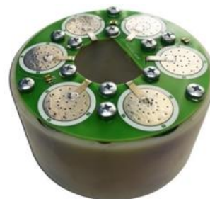
Figure 22. Battery module assembly
