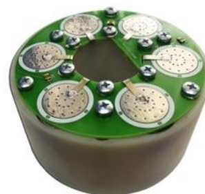
Figure 22. Battery module assembly
