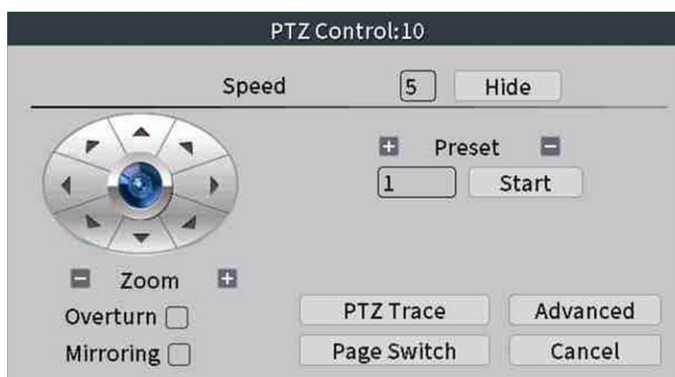
Figure 25. PTZ Video Camera control panel
