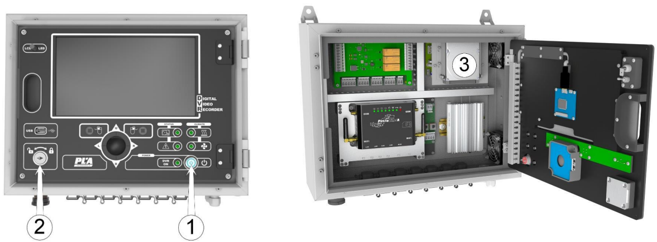
Figure 44. Replacement of the removable memory drive of the DEL-150V3-MDT4 Video Recorder
