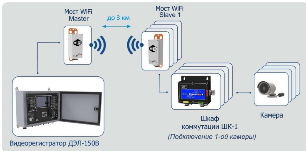
Figure 30. Example №2 DEL-150V2 diagram connection
