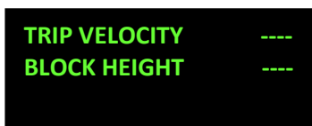
Figure 10. Readings in case of loss of communication with the DPS-140
