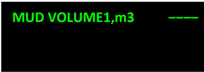
Figure 13. Readings in case of loss of communication with the U-150
